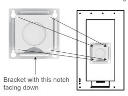
3 Lock the holes aligned in step two one by one with short screws.
