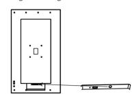
② Place the side of the bracket with the groove facing downwards, then align the four small round screw holes (the four holes inside) on the bracket with the four holes on the digital calendar.
